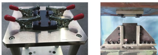
(a) Low velocity impact test fixture (b) Compression test fixture
