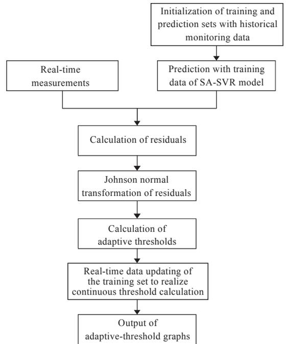
Fig. 5 Flow chart of the dynamic adaptive threshold model
