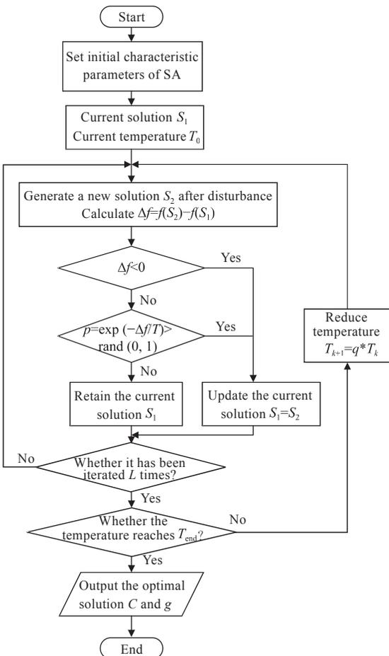
Fig. 2 Flow chart of the SA algorithm
