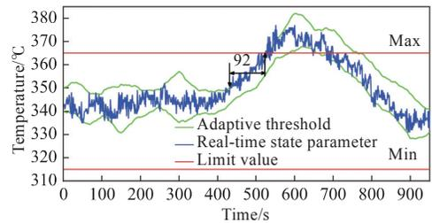
Fig. 7 Verification of abnormal data in the dynamic adaptive threshold model
