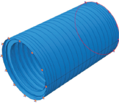
Fig.8 Boundary conditions of cylindrical shell FE model
