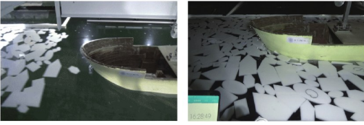
Fig. 6 Ship model entering the ice field (left) and its interaction with ice blocks when sailing in ice field (right)
