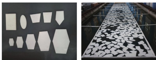
Fig. 5 Brush ice blocks (left) and corresponding random ice field (right)
