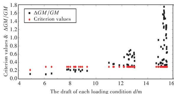
Fig.1 The first level criterion results of parametric roll
