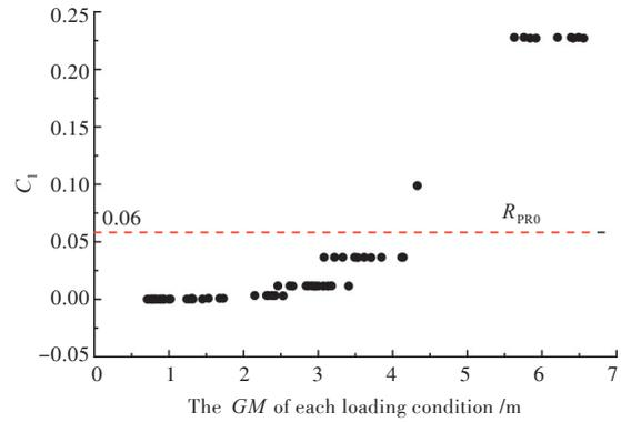
Fig.3 The second level criterion 1<sup>st</sup> check results of parametric roll
