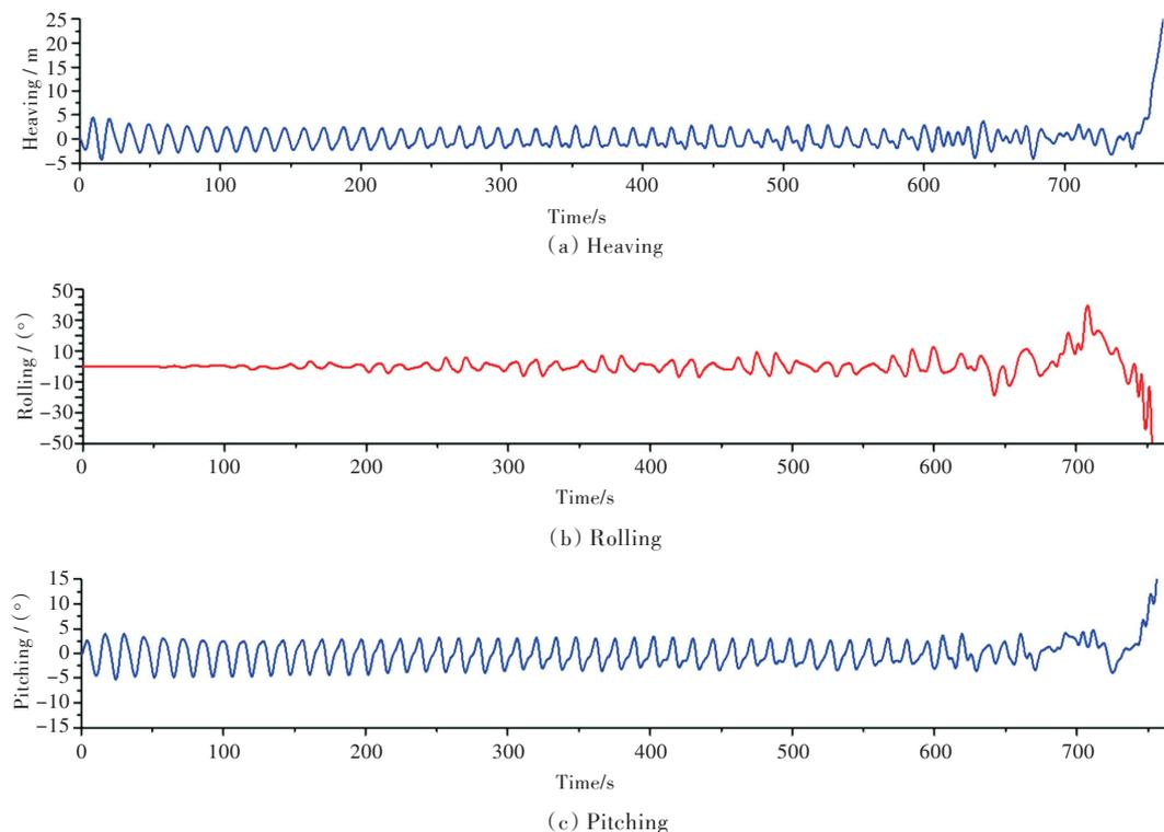
Fig.7 Time history curves of heaving,rolling and pitching at condition II -6
