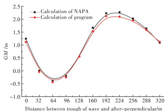
Fig.5 Variation of  $GM$  with hull and waves' relative position
