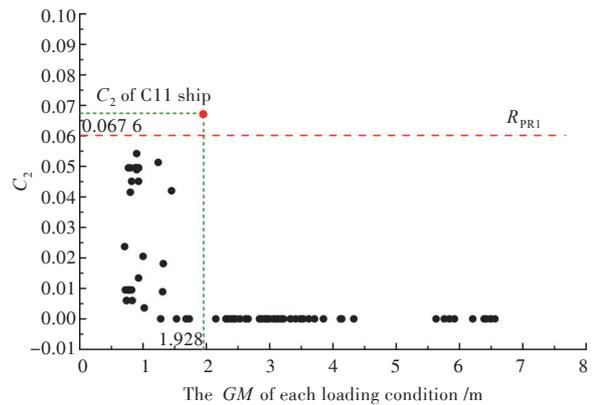
Fig.4 The second level criterion 2<sup>nd</sup> check results of parametric roll
