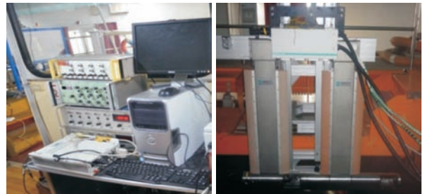
(a) Torque and angular displacement data collection system (left) and underwater PIV measuring system (right)
