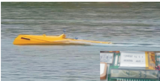
(b) \Omega -type freeboard (free-running speed of model is 9.2 m/s)
