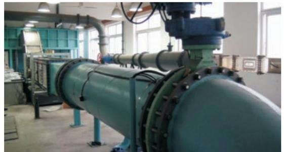
Fig.12 Gravitation water tunnel
